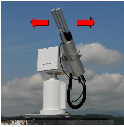
When the airmass went below the threshold (4.5), scattering angle will be 180 deg., and direction of the scattering scan will be normal movement of;
