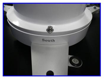
4. Adjust the horizontality of the skyradiometer by using a water bubble on the leg of sun tracker. It is necessary to maintain the sun tracking accuracy.
