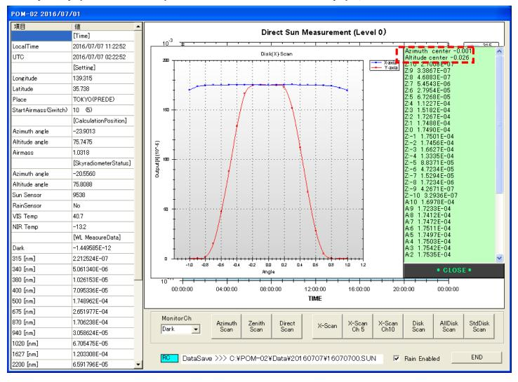
X-Scan is the process to align the optical axis. This process is recommended when the skyradiometer was relocated and re-installed. Adjust the values of Azimuth center and Altitude center within +/- 0.050, by the screws. Please adjust both at Ch5 and Ch10.
