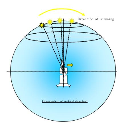
Scattering angle : Max. 24 points (Depending on the calculation of the scattering angle) 0,2,3,4,5,7,10,15,20,25,30,40,50,60,70,80,90,100,110,120,130,140,150,160
