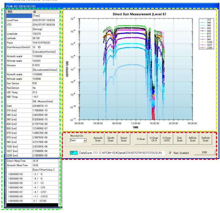
: Graphic display of direct beam measurement data, since the observation program has started.
