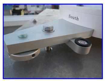
NOTE: It is necessary to fix skyradiometer to the flat and robust mounting base, for the fall-prevention against the strong wind.
