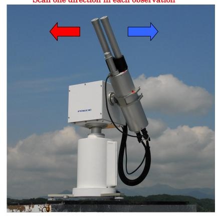
When the airmass exceeded the threshold (4.5), scattering angle will be 30 deg., and direction of the scattering scan will be normal movement of;
