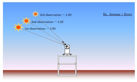
4. Direction of Aerosol observation: Observes horizontal direction of east and west alternately.
