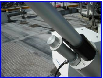
11. Make sure that the sun light is on the center of the target.
