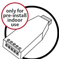
A type of USB-RS485 converter that supports half duplex 2-wire connections and preferably has optical isolation for increased safety and reliability.
