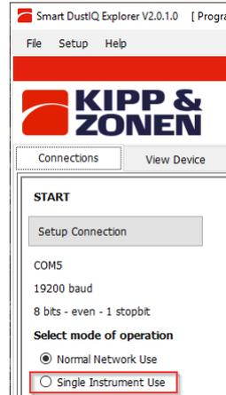
Go back to the first Connections tab to change to Single Instrument Use when the baud rate or parity needs to be changed too. Modbus address changes work also in Normal Network Use.
