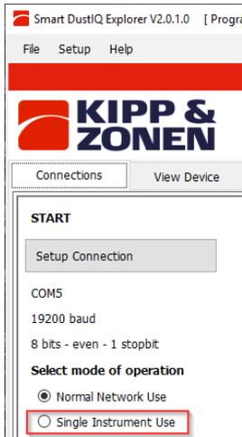
When the communication parameters are known and properly setup and only the Modbus ID is unknown a Send Broadcast will find the attached DustIQ and show it.
