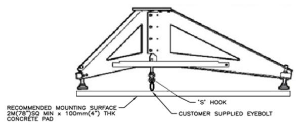
Figure 12 Securing the Tripod
