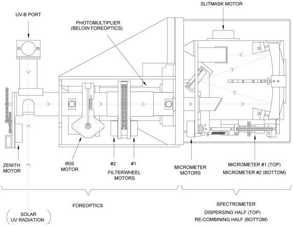
Figure 6 Top view of spectrometer
