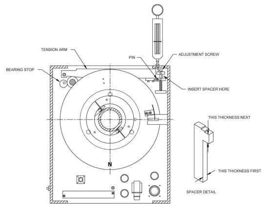
Figure 14 Tracker drive mechanism
