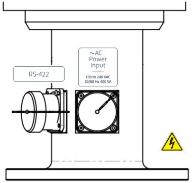
The RS-422 connector is the communication connection input.
