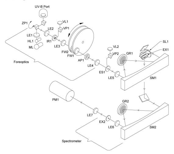
Figure 5 Optical Elements of Brewer Spectrophotometer
