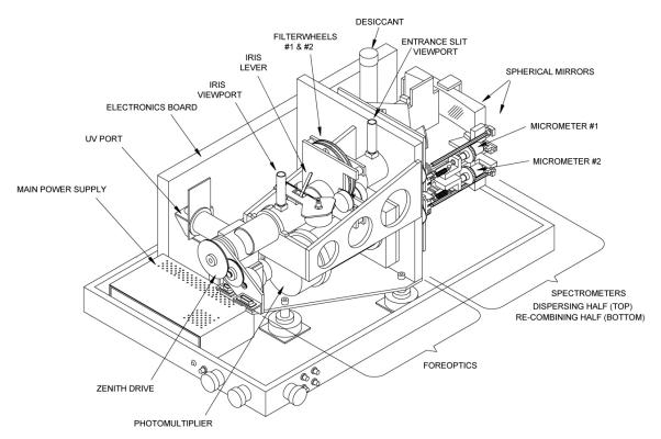
Figure 3 View of the Brewer with the top cover removed
