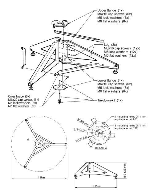
Figure 10 Brewer Spectrophotometer Tripod
