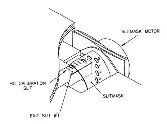
Figure 8 Slit Mask Assembly
