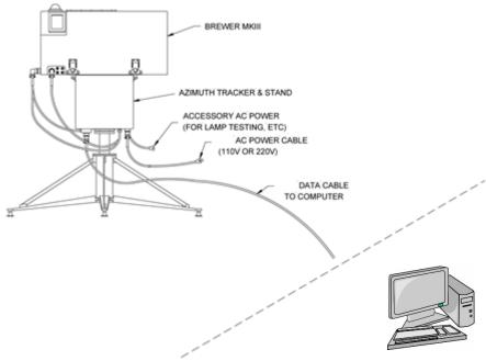
Figure 9 Brewer Equipment Setup
