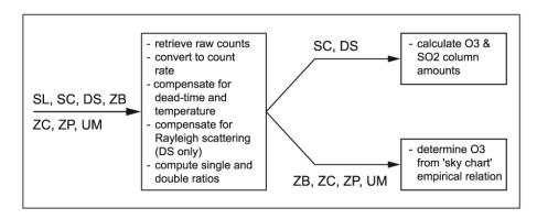
Figure 15 Data Reduction Flowchart
