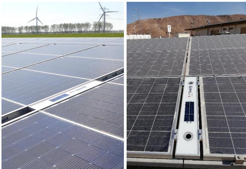
If the DustIQ is installed on a support structure it is advised to use the same end-clamps as you would for 35mm high PV modules. The supplied clamps are not meant to be used as an end-clamp.
