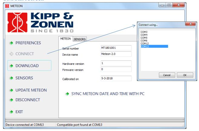
The bottom line of the start screen shows if a Meteon is found on one of the available COM ports, if not, the sub-menu [Connect using..] offers the option to pick one of the available COM ports by hand.
