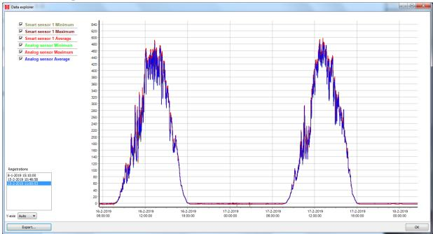
When downloading the data from the METEON it is visualized with the above Data Explorer screen.
