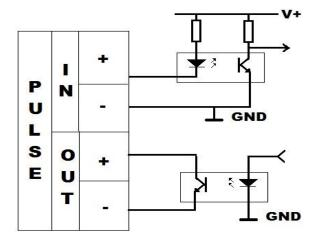
The SO outputs (often called SO+, SO- or S+ and S-) have to be connected to the Pulse input of the Meteon. Both pulse in- and output are optically isolated. The input can be tested by connecting the + and – inputs to simulate an input pulse. The picture on the left shows a simplified schemeatic of the inside of the Meteon.
