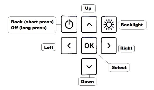
The On/Off – Back key will turn on the Meteon after a short press and turn off after a long press (>1 second, and only when in top level menu). When on, a short press will go one level up.
