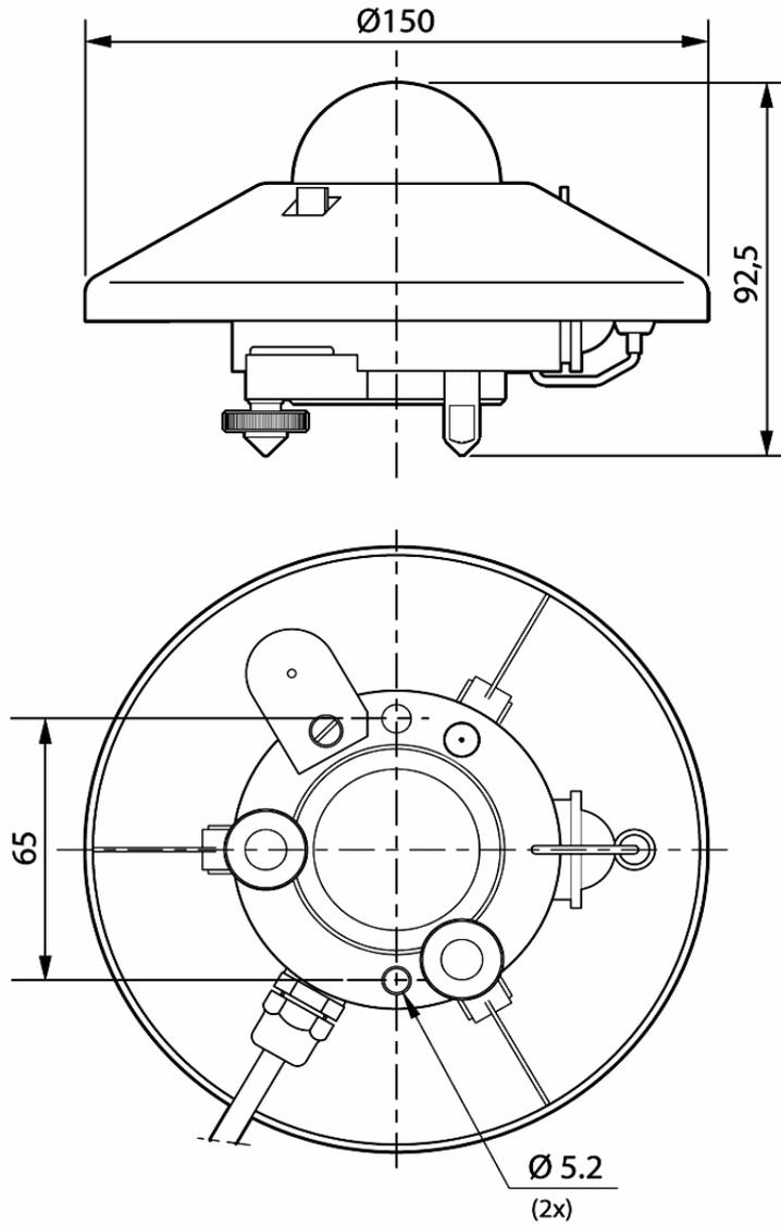
Figure 2 CM 21 Pyranometer outline dimensions in mm.
