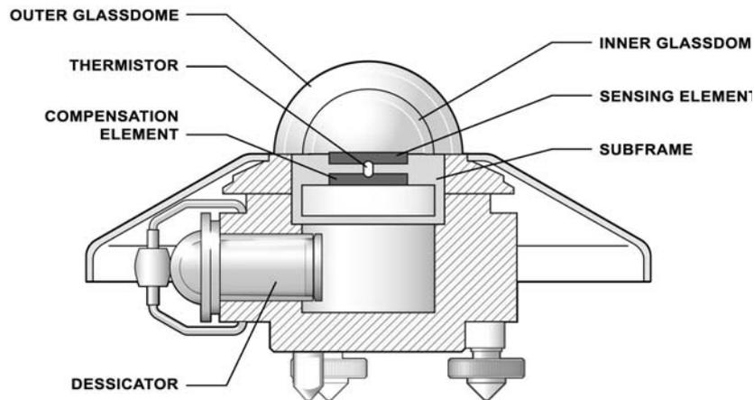
Figure 1 Construction details of a CM 21 pyranometer
