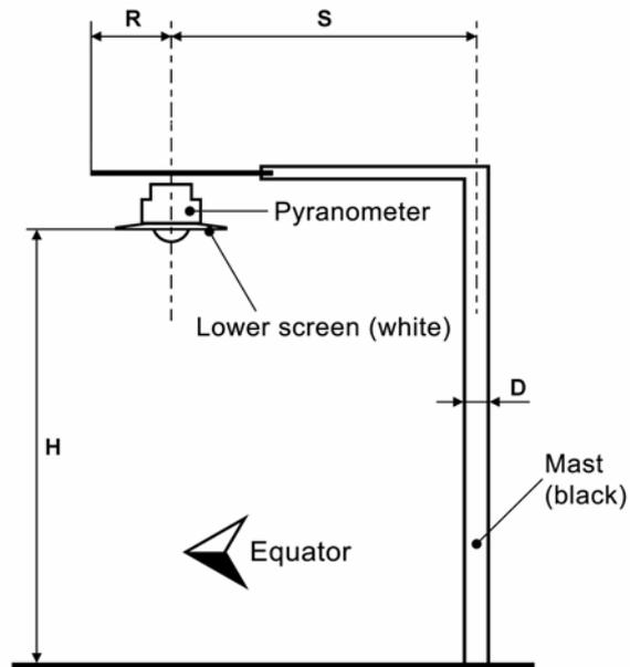
Figure 8 Arrangement to measure reflected global radiation
