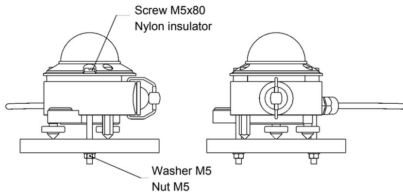
Figure 7 Mounting the pyranometer.
