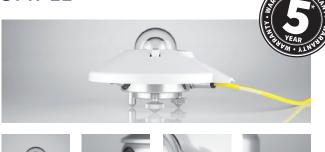
SMP11 has the same housing and detector design as the passive CMP11 model and is an ISO Secondary Standard pyranometer. Like SMP3 and SMP10, the SMP11 is equipped with a smart interface and there are two versions, One has an analogue output of O to 1 V, the other has 4 to 20 mA. Both
