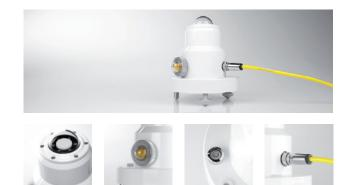
UVS instruments have a precision quartz dome and specially shaped diffuser to provide class-leading directional response. The detection system includes optical filters, a very sensitive phosphor and a photo-diode. The system is temperature stabilised at +25 °C ( $\pm$ 2 °C) to prevent changes in spectral response and sensitivity with variations in the ambient conditions. The signal output is amplified and the internal stabilisation temperature can be monitored.
