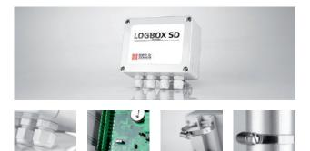
**LOGBOX SD** is an 8 channel data logger that allows connection to multiple instruments at the same time. Each input can convert measured values into the correct engineering units. The data is stored on the internal 128 kB memory or the 512 MB SD memory card that is included as standard.
