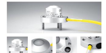
SP Lite2 is designed for all-weather measurement of solar radiation. It has a specially shaped diffuser that gives very good directional response and is largely self-cleaning. The detector is a silicon photo-diode, so the spectral response is not as broad or flat as our CMP/SMP series pyranometers with thermopile detectors.
