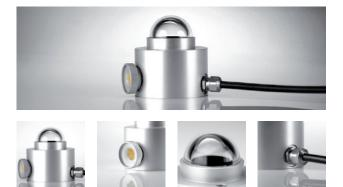
CM4 is a high temperature pyranometer for measuring solar or artificial light irradiance under the most extreme temperature conditions. With an operating temperature range from -40 °C to +150 °C and measurement up to 4000 W/m<sup>2</sup> it is a unique instrument. All the radiometer components are specially selected for their ability to withstand these extremely high temperature and irradiance levels.
