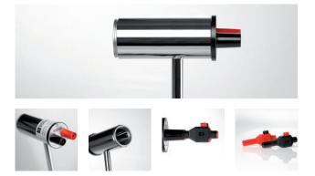
CA2 is based on the same type of thermopile detector as our CMP3 and CMP6 pyranometers. Because it has a limited field of view it can be used to measure the intensity of radiant fluxes coming from a specific location or a specific source.
