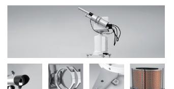
**POM-O1** is a sky radiometer mounted on a dedicated sun tracker. It uses a single detector and rotating filter wheel to measure radiation in seven narrow wavebands, either directly from the sun or at user-defined angles away from the sun. The instrument has a base with levelling feet and a sun sensor for active tracking of the sun position. Installation is quick and simple and a precipitation sensor is included so that the radiometer is pointed downwards during rain to keep the optics clean.
