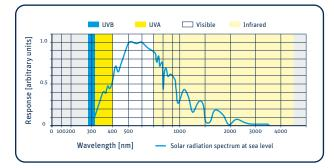
The amount of UVB and UVE radiation reaching the ground is strongly dependent upon altitude, the height of the sun in the sky, the amount of Ozone in the atmosphere and cloud cover. UVS radiometers are calibrated for a typical air-mass (solar zenith angle) and Ozone column concentration. Our unique UVIATOR software supplied with the UVS further improves the accuracy of the measurements by correcting for the amount of Ozone in the atmosphere and the solar elevation.
