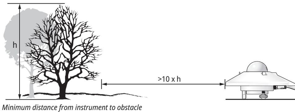
The minimum distance is important for measuring the direct radiation. The diffuse solar radiation is not so affected by obstacles near the horizon. An obstacle to the field of vision that rises 5 degrees over the entire azimuth range of 360 degrees reduces the diffuse radiation directed downwards by only 0.8%.
