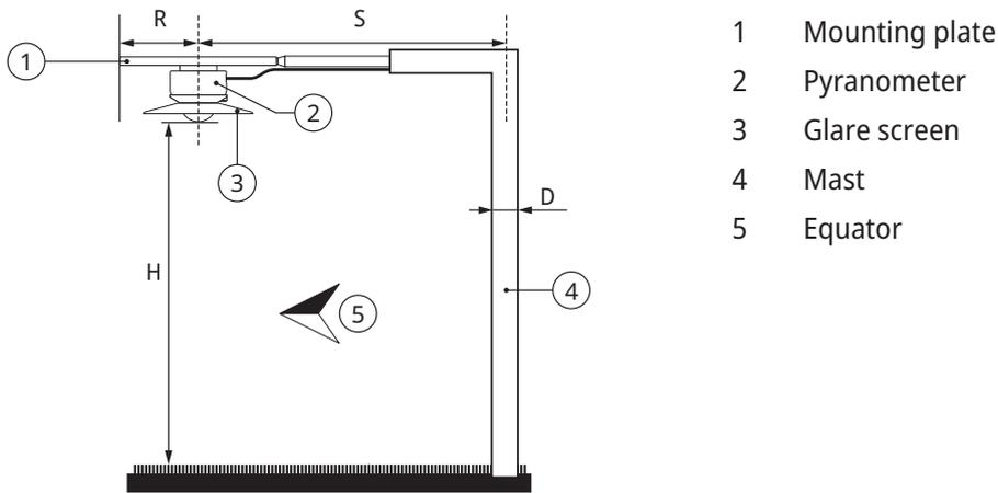
The mounting plate prevents the pyranometer from being heated by solar radiation. The optional glare screen has an angle of 5 degrees and prevents direct radiation on the glass dome during sunrise and sunset.
