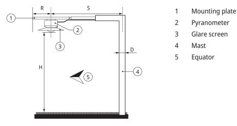
The mounting plate prevents the pyranometer from being heated by solar radiation. The optional glare screen has an angle of 5 degrees and prevents direct radiation on the glass dome during sunrise and sunset.
