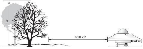
Minimum distance from instrument to obstacle
