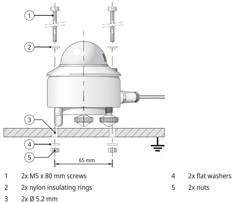
• To insulate the instrument against the temperature of the mounting device, place the instrument on the adjustable foot and the two leveling feet.
