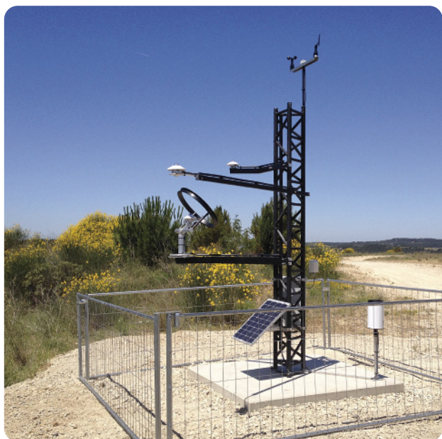
Station with global, diffuse and reflected radiation measurements and albedo
