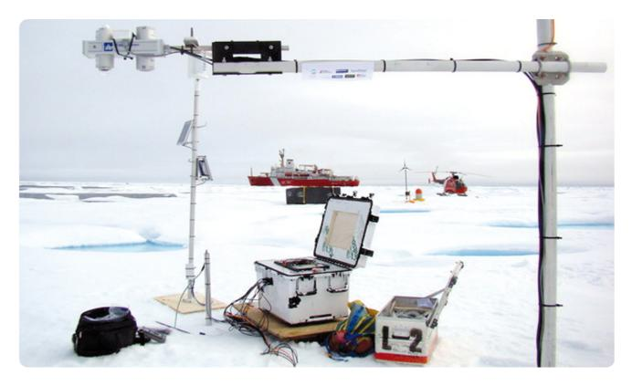
To quantify the energy balance David needed to measure incoming and reflected solar radiation, down-welling and up-welling far infrared radiation and to calculate albedo and energy fluxes. For this he required a high quality, reliable instrument with proven performance in polar conditions. Like many other scientists involved in research in Polar Regions and on glaciers, David chose the Kipp & Zonen CNR 1 net radiometer as a key component of the SAMS monitoring package.
