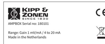
The standard AMPBOX gain setting is 2 mV/mA, so that 0 to 32 mV input gives 4 to 20 mA output
