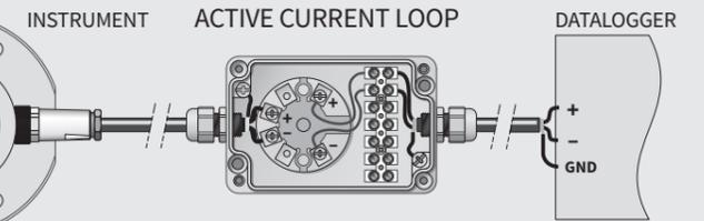
The current loop has to be powered with a supply, or active receiver, capable of providing 7.2 V for AMPBOX plus sufficient for the loop cable voltage drop. Maximum 35 V
