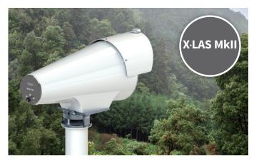
Path-averaged measurement of turbulence and sensible heat fluxes, 1 second response time
