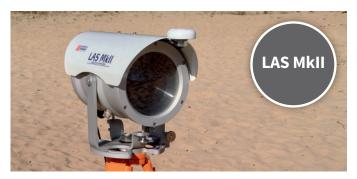
Remote measurement by Large Aperture Scintillometry
