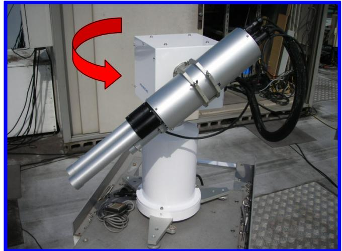
**NOTE:** Connectors of rain sensor, power cable, and communication cables are screw type, so that please make sure all connectors are tight enough.
