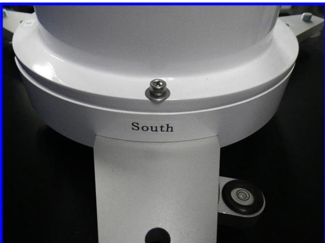
4. Adjust the horizontality of the skyradiometer by using a water bubble on the leg of sun tracker. It is necessary to maintain the sun tracking accuracy.
