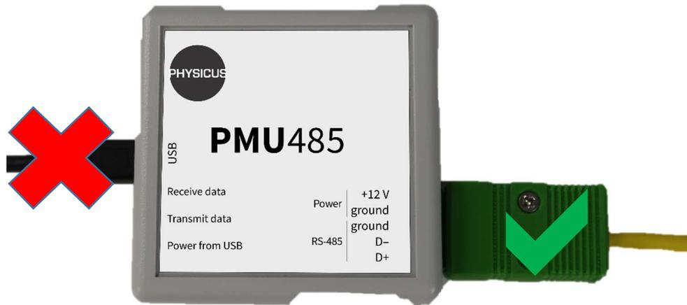
Unplugging the USB connector interrupts the computer's serial communication abruptly and could cause the used RS-485 or Smart Explorer software to crash.
