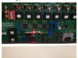
A.Start the BrewCMDW utility and observe that the instrument has responded and note which mode is indicated. The program should display the same mode as the mode observed on the status LED.
