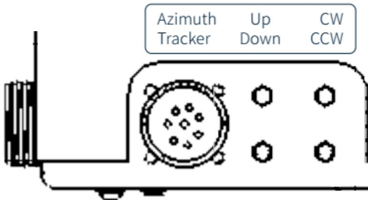
The azimuth tracker connector is the tracker operation cable connection input.
