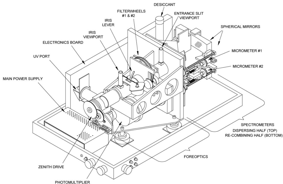
Figure 3 View of the Brewer with the top cover removed
