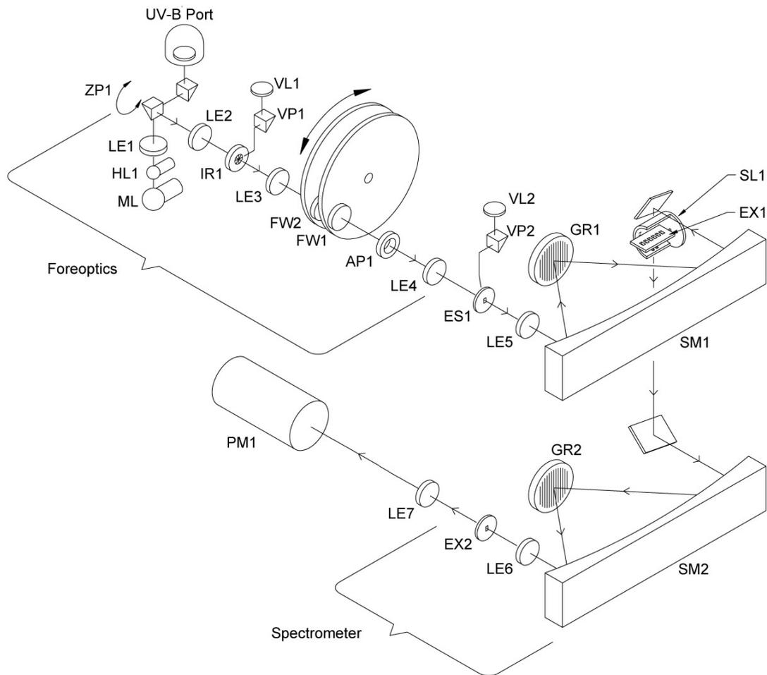
Figure 5 Optical Elements of Brewer Spectrophotometer
