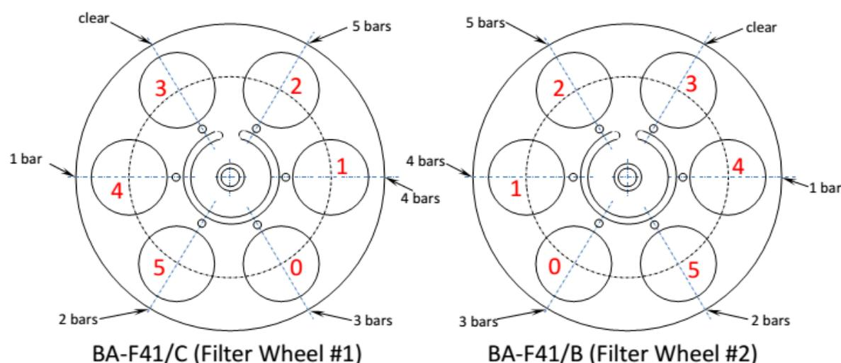
Figure 7 Diagram of filter wheels
