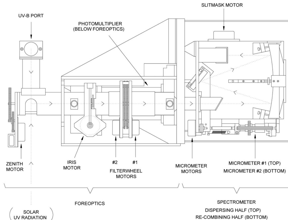
Figure 6 Top view of spectrometer
