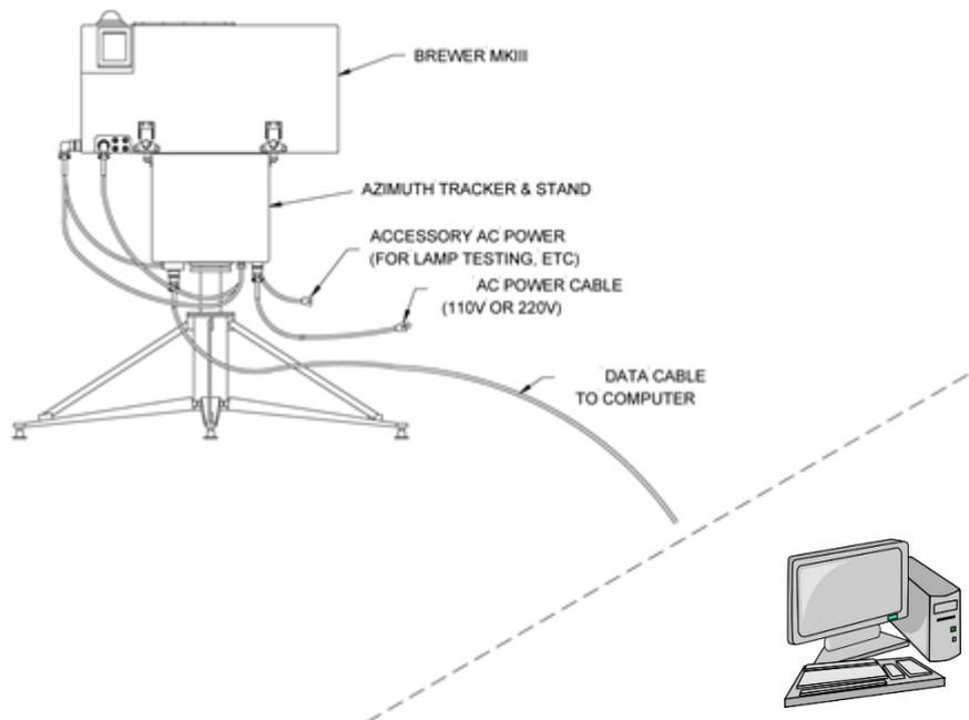
Figure 9 Brewer Equipment Setup
