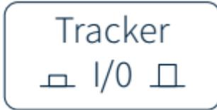
When button is flush with the housing the power is off.
