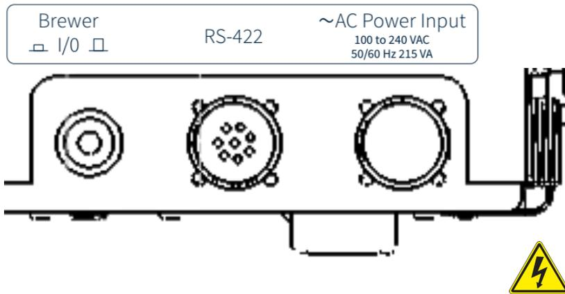
The RS-422 connector is the communication connection input.
