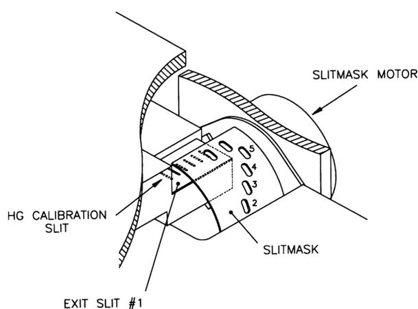
Figure 8 Slit Mask Assembly
