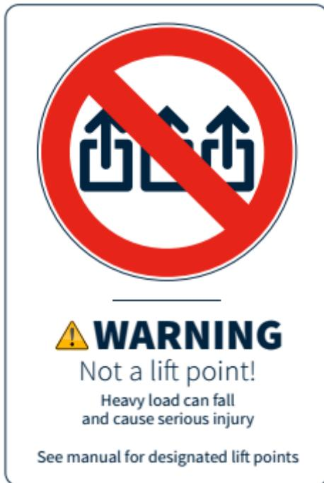
Do not lift the complete instrument using the handles.
