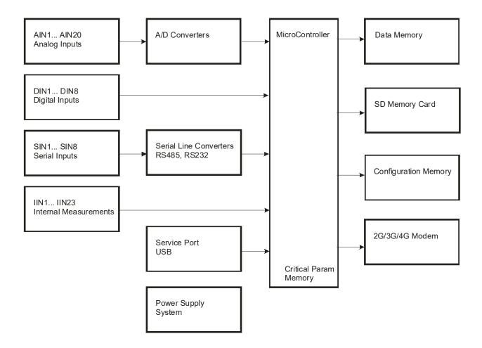
Datalogger block diagram shows most important blocks. In respect to security assessment, there are 4 communication ports available for the user: COM1 (RS485 or RS232), COM2 (RS232), USB service port and Modem. COM 1 is reserved to communication with external serial sensors and it is not possible to access datalogger service mode.
