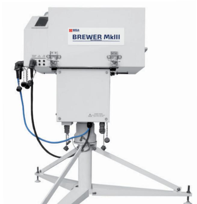
An internal fan, heater and humidity sensor are fitted as standard.
