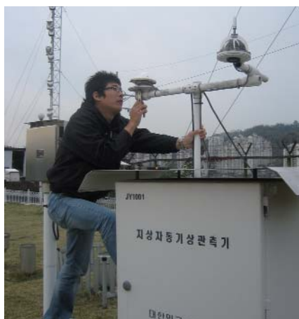
Y.K. Kim, B&P Engineer, installing a CMP 21 on a Synoptic Weather Observation Station
