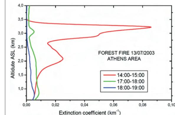
Figure 3. Evolution of forest fire smoke measured with a LB-Series LIDAR
