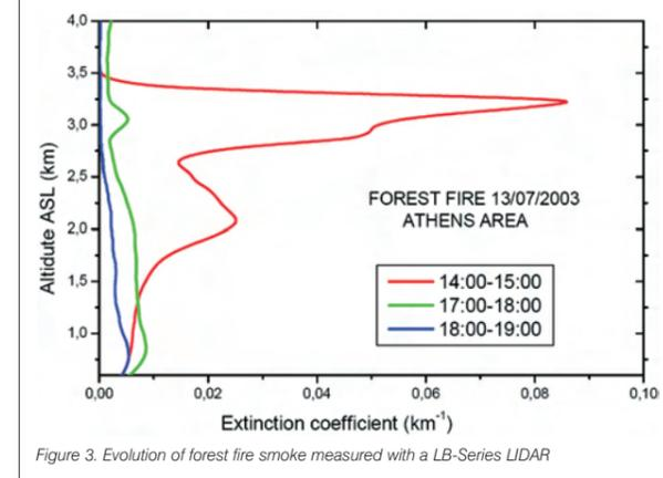
Figure 3. Evolution of forest fire smoke measured with a LB-Series LIDAR
