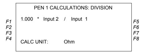
The result of the calculation, the resistance measured, is now written to Pen 1. It is possible to show the resistance value directly in enlarged digits on the screen. To do this select the function: **DISPLAY ENLARGED PEN 1**.
