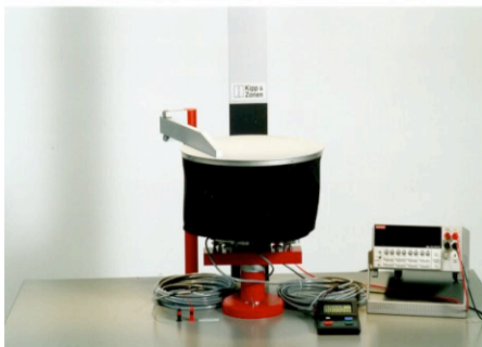
figure 8 Different positions of the turntable and shutter during the calibration procedure
