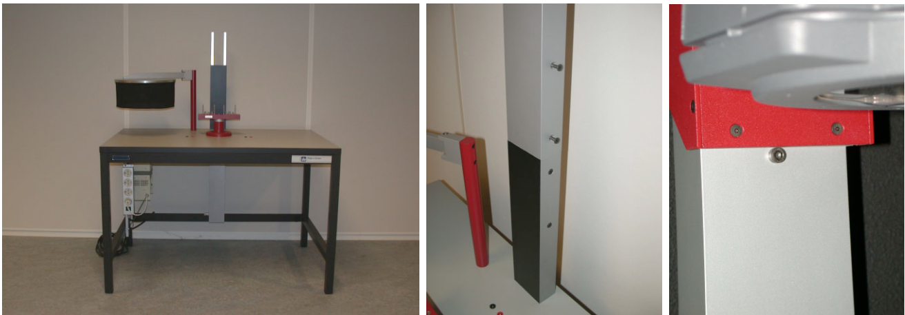
figure 1 Calibration table with lamp pillar
