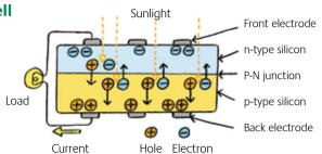
"Yes, indeed. When the solar cell receives sunlight, negative electrons inside move to the n-type silicon and holes gather at the p-type silicon. This means electricity has been made. Now, go ahead and see if it supplies electricity to run this pump."
