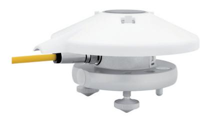
**CGR 3** is the partner to the CMP 3 pyranometer. It has a flat silicon window which provides a field of view of 150°. The small size and sealed construction make this instrument the ideal choice for horticulture and agriculture. A screw-in mounting rod is available for easy installation.
