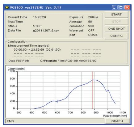
The intensity is not affected, but the noise is significantly reduced. However, when measuring natural sunlight, if too many averages are made the atmospheric conditions may be changing during the process.
