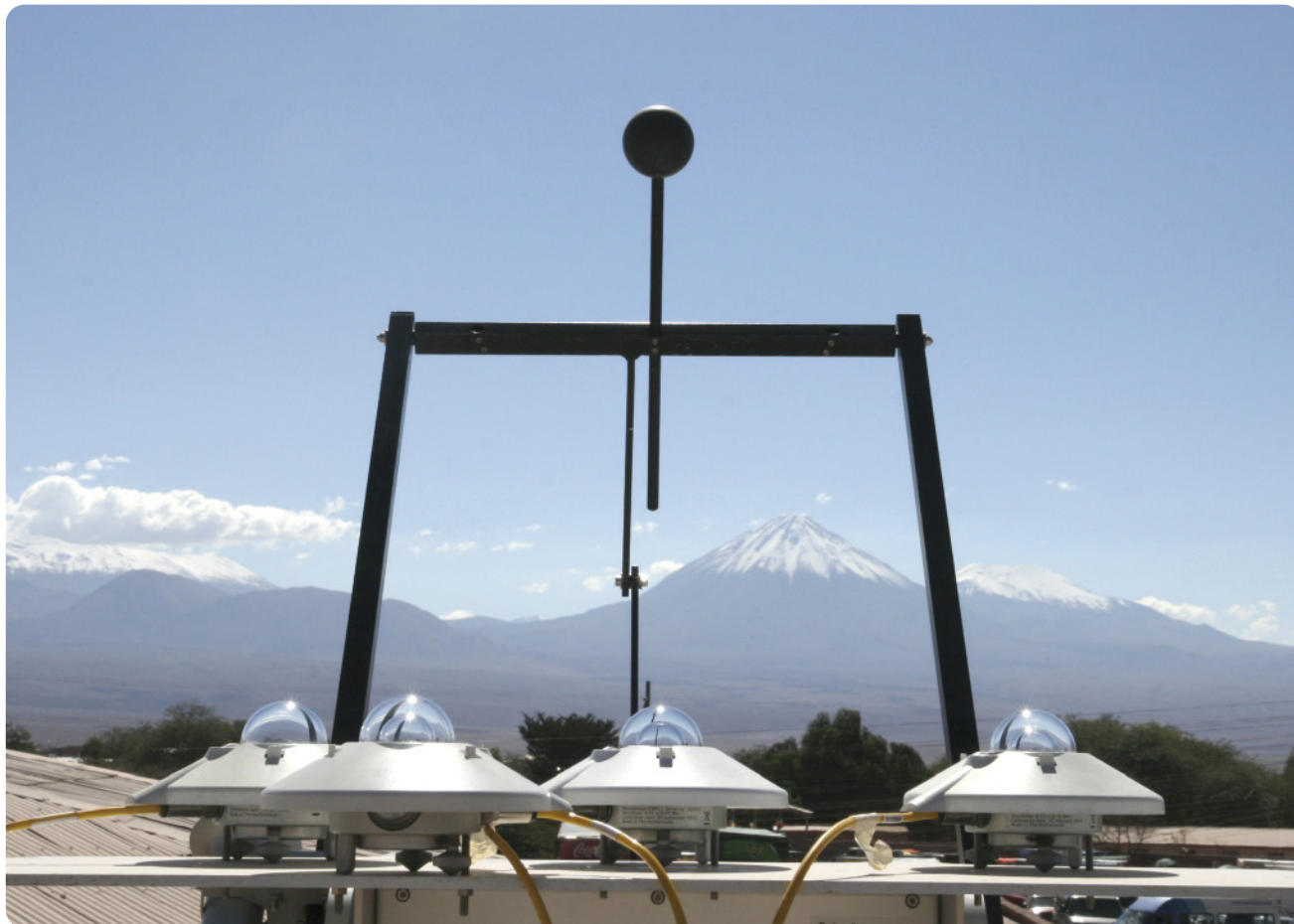
SOLYS 2 sun tracker at the PUC station, installed in 2010 at San Pedro de Atacama, in the Chilean desert
