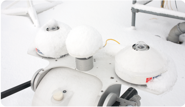
From the left: CMP 21 ventilated without heater, CMP 21 unventilated, CMP 21 ventilated and heated
