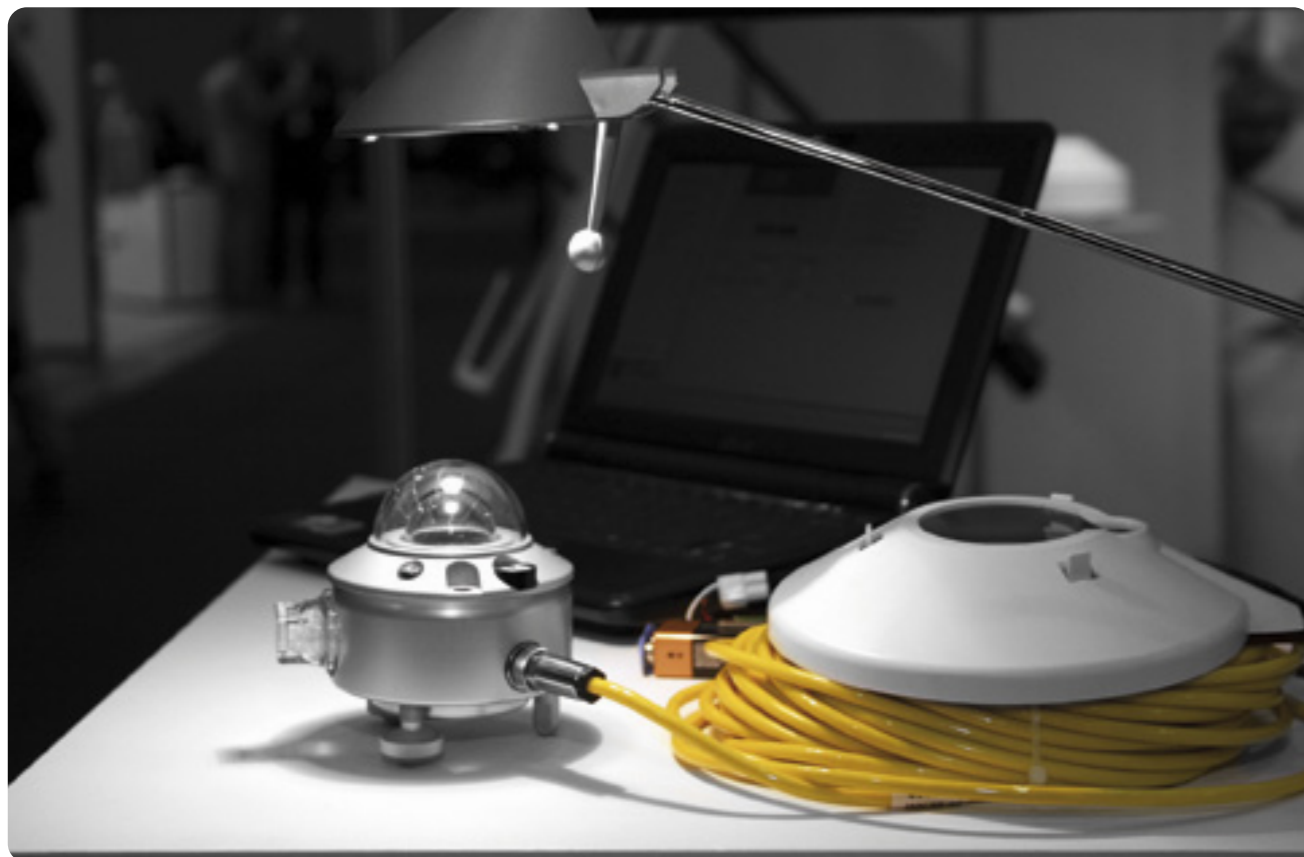
SMP11 on display at Meteorology Technology World Expo: A halogen lamp over the pyranometer resulted in a display of more than 700 W/m 2
