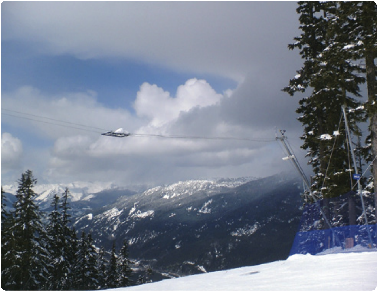
Figure 2, the suspended instrument platform above the Dave Murray downhill course and instruments on a tower to the side of the ski run
