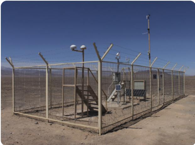
*A typical Mainstream solar radiation measurement station*
