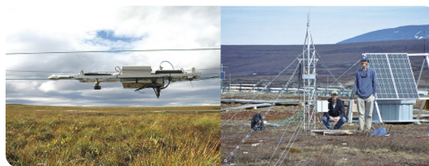
Left: CNR 4 Net Radiometer at far left of sensor system on support cables at Toolik Lake, Alaska
