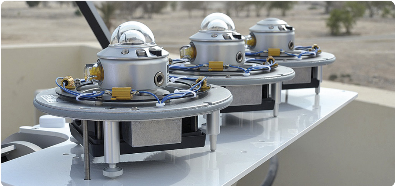
The CMP 11 pyranometers and CGR 3 pyrgeometer being fitted on a CVF 3 ventilation unit before the cover is mounted
