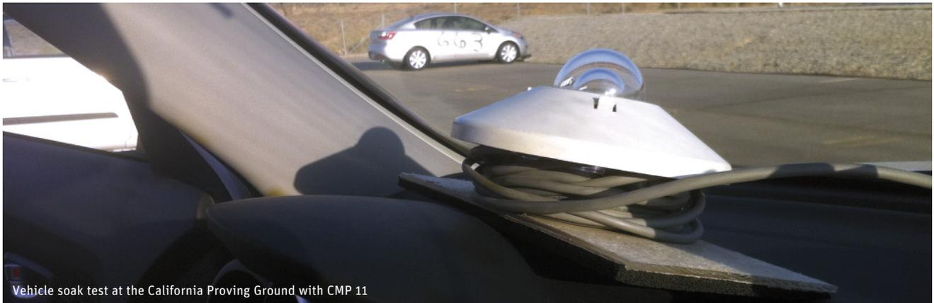
Vehicle soak test at the California Proving Ground with CMP 11
