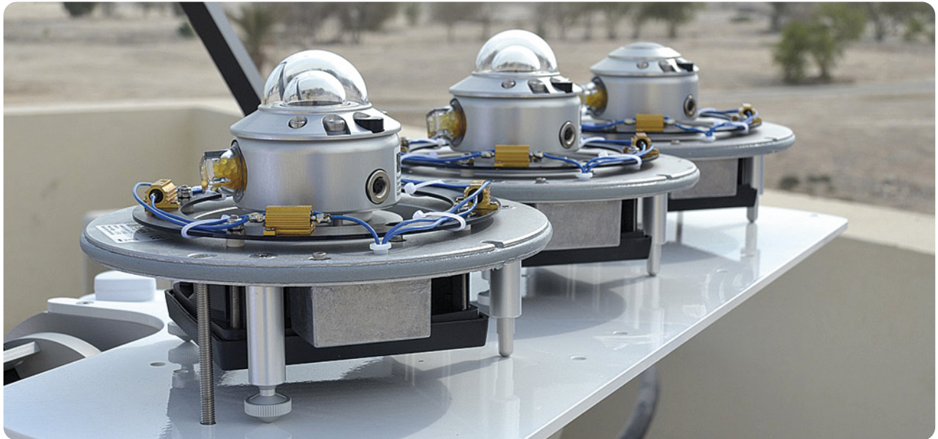
The CMP 11 pyranometers and CGR 4 pyrgeometer being fitted on CVF 3 ventilation units before the covers are mounted
