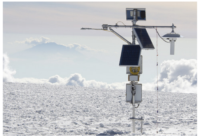
CNR 4 to left, temperature and humidity sensors to right Mount Meru 70 km in the background
