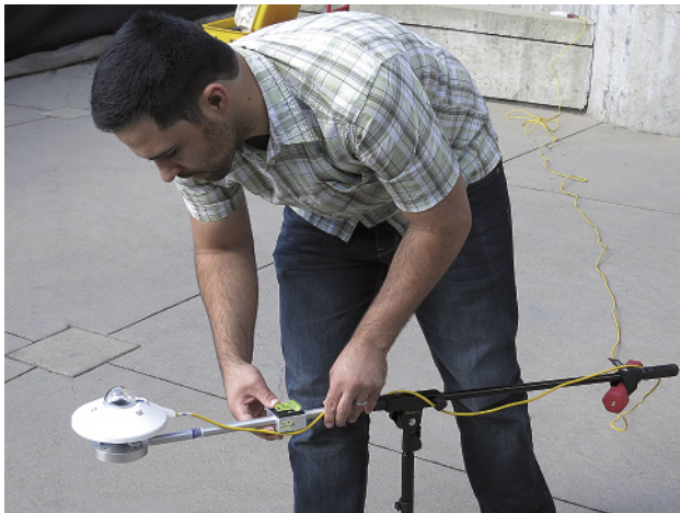
Mounting rod has two cross-levels, one for the CMP 6 facing up, the other when facing down
