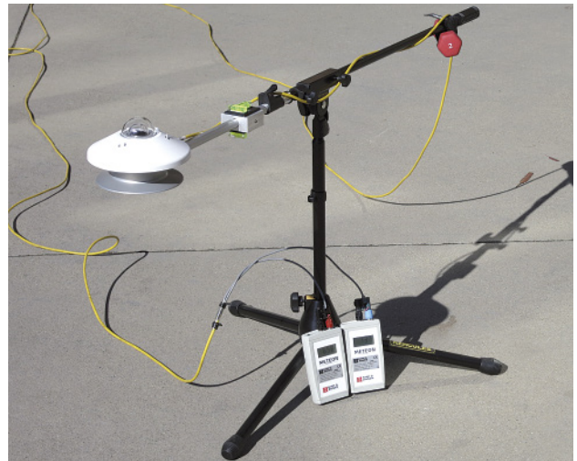
CMA 6 with two METEONs, which are normally positioned out of view of the lower sensor
