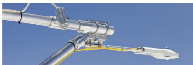
Until our CNR 4 was installed in 2012, we measured each radiation component separately; engineering considerations required situating instruments close to the tower, which influenced measurements. Now, with the lightweight CNR 4, our measurements are being made further from the tower and better represent the four variables. During fieldwork at the site leveling adjustment consumes far less time than is required to level four different instruments.
