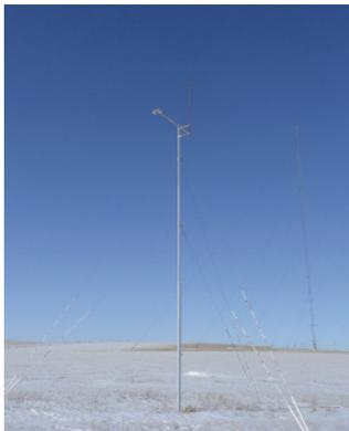
meteorological tower that includes a CNR 1 net radiometer. With the addition of ventilation units to the downwards facing radiometers the site will comply with the requirements for an Extended Baseline Surface Radiation Network Station (BSRN).
