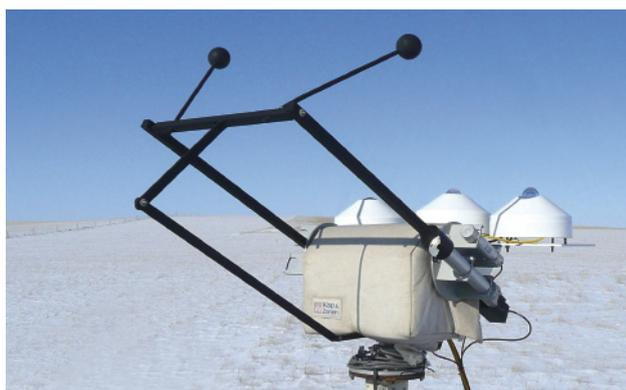
The trackers are fitted with CHP 1 pyrheliometers, CMP pyranometers and CGR 4 pyrgeometers; to measure direct, diffuse and global short-wave radiation and downwards long-wave radiation. An additional pyranometer and pyrgeometers measure reflected short-wave radiation and upwards long-wave radiation. All the pyranometers and pyrgeometers are fitted with CVF 3 ventilation units.
