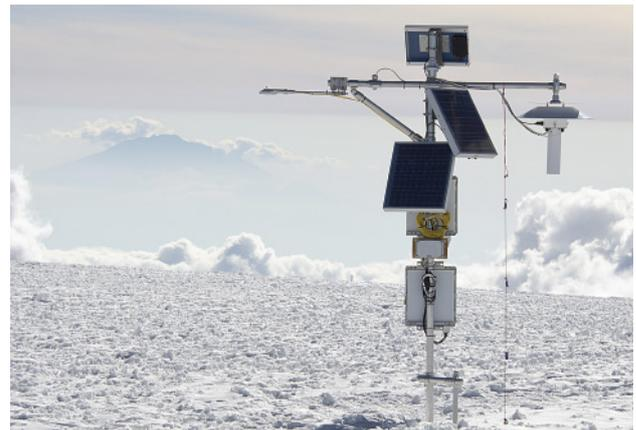
*CNR 4 to left, temperature and humidity sensors to right
