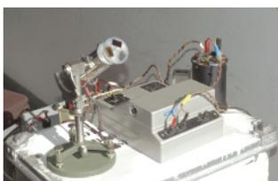
We had purchased this to replace the old Angstrom pyrheliometer, which had not been calibrated for decades. In addition it took dedication from the observer to produce results, as a single observation needed many adjustments and the readings could take half-an-hour to complete. As a consequence observations had been made relatively infrequently at Rothera, and indeed most of them were made during my occasional visits.
