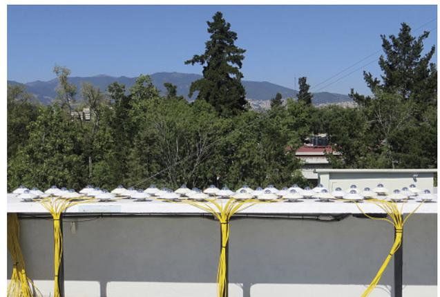
CMP 11 field pyranometers for AWS being calibrated at UNAM
