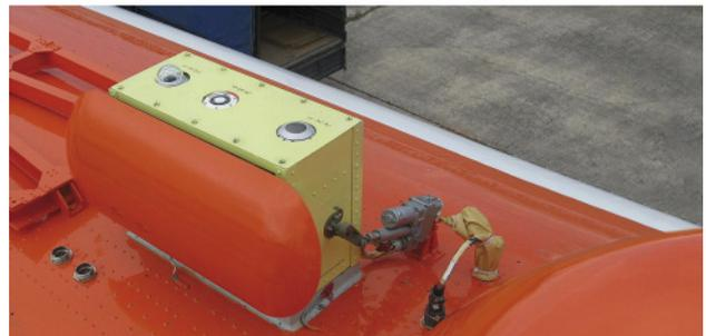
*View with fairing removed: rack with radiometers and the retractable cover. (Photo: Roshydromet)*
