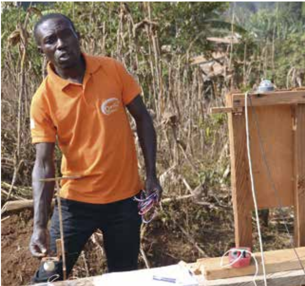
Staff member Collins, showing the measurement setup in Tatum. The CM 5 pyranometer, a digital air thermometer and a ping-pong ball functioning as a wind velocity indicator
