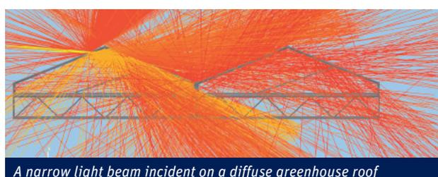
A narrow light beam incident on a diffuse greenhouse roof
