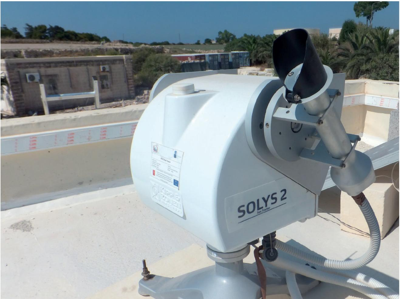
The SOLYS2 with CHP1 pyrliometer on the roof of the Institute for Sustainable Energy
