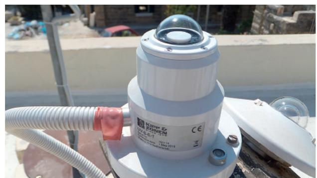
*The Kipp & Zonen UVS-E-T UV Radiometer*
