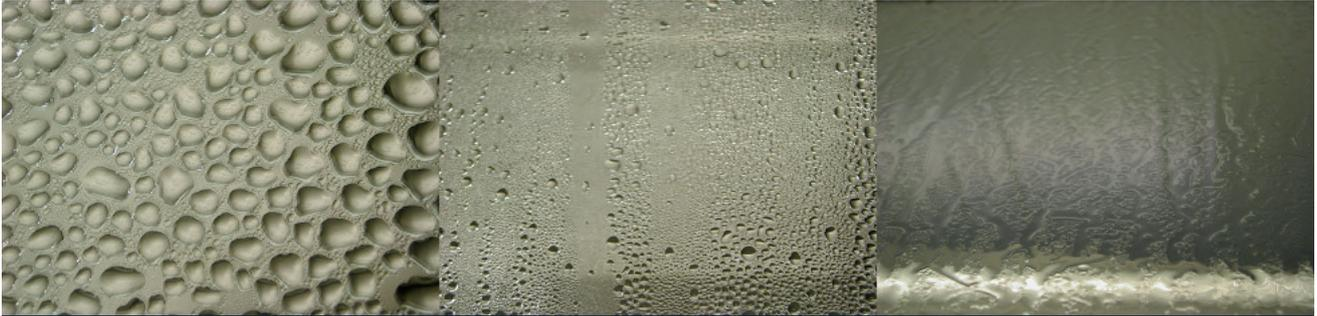
*Condensation on glass surfaces with different hydrophobic or hydrophilic surface properties*
