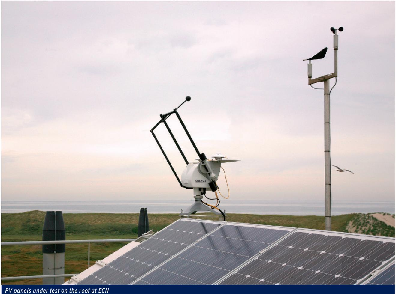
*PV panels under test on the roof at ECN*
