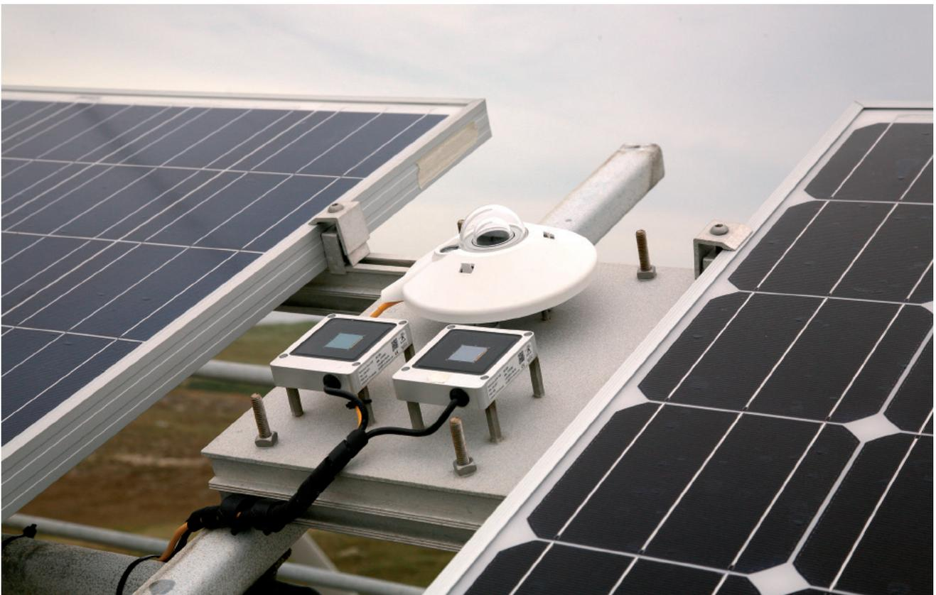
Plane of Array pyranometer and reference cells
