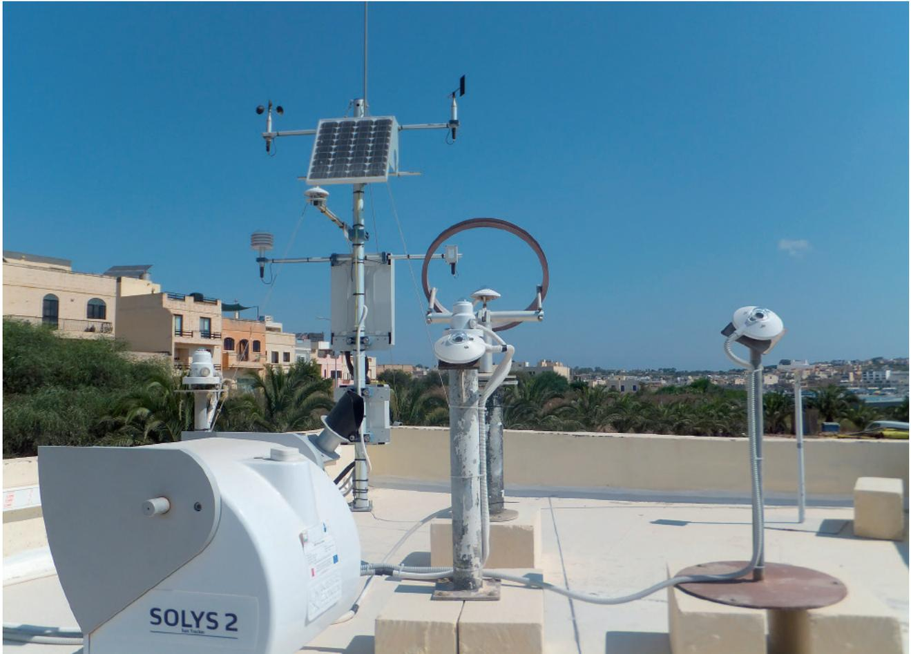
*The complete solar and meteorological monitoring station on the roof of the Institute for Sustainable Energy*
