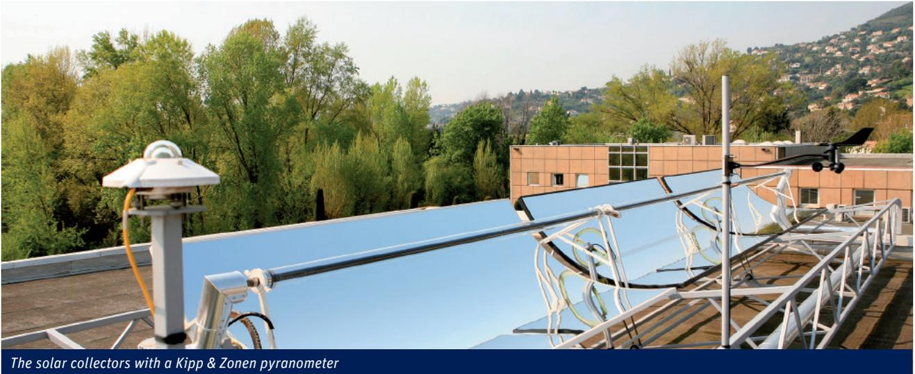
*The solar collectors with a Kipp & Zonen pyranometer*
