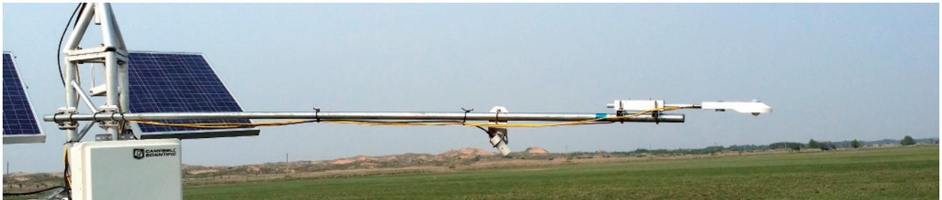
The system integrates a wheeled platform, measurement equipment, autonomous power supply unit, recording and data analysis equipment into one complete machine. It can collect, analyse and store output parameters, such as energy fluxes, corresponding data quality information, the details of the source region and environmental factors required by ecological system models.
