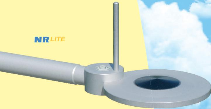
NR Lite is a low cost net radiometer with a Teflon™ coated, weather resistant black conical absorber. A vertical stick prevents birds from affecting the measurement. NR Lite is based on a single differential thermopile sensor and has one output for the total net radiation.
