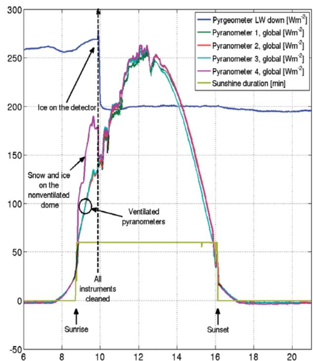
This initial review of the case study results demonstrates the necessity of using a ventilation unit and heating with pyranometers in Finnish winter conditions ■
