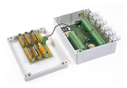
Last step is to connect the supplied USB cable with the computer. The LOGBOX SE Setup software can be used to setup the logger and related sensors. Do not switch the LOGBOX SE on yet. The USB connection or 6 AA batteries can both supply the board enough electrical power to perform the setup.
