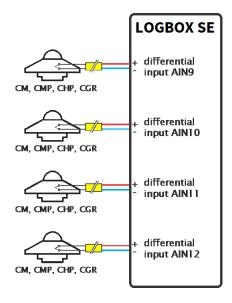
The LOGBOX SE allows you to connect up to 4 sensors on the differential analog inputs AIN9 to AIN12 which have a selectable input from 19mV up to 2500mV.
