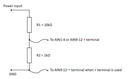
Input range 2500mV for the differential inputs.
