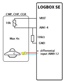
In the illustration the 10K thermistor is connected to AIN 1 but in practice it can be connected to any of the four analog single ended inputs AIN1 – AIN4.
