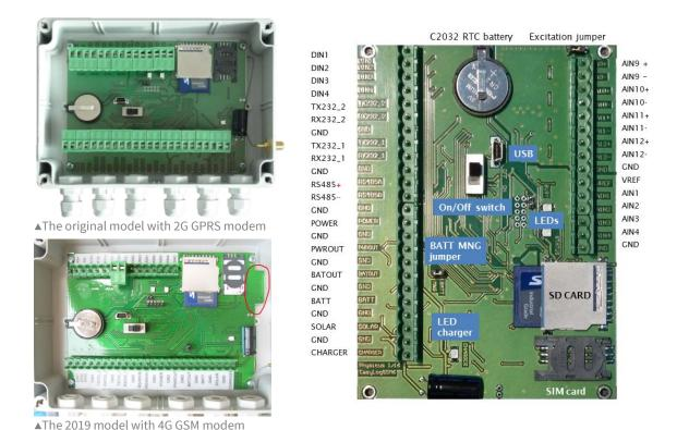
Thanks to clear layout the user can easily connect relatively large number of sensors. For better access to input connections, connectors are divided by two or three and removable.
