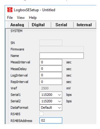
Using LogboxSESetup 1.9 and above the RS485 address was set to 2.
