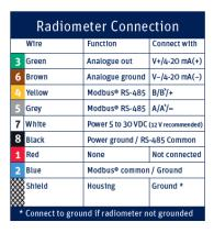
The sensors need constant power to stabilise and to be able to provide fast response to irradiation level changes.
