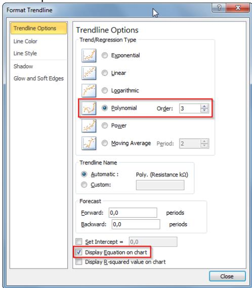
**Step5:** The result will be as below with a text box with the polynomial as calculated by e.g. Excel. It has been moved and made red here to be better visible.
