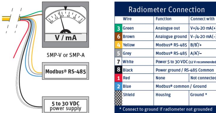
The sensors need constant power to stabilise and to be able to provide fast response to irradiation level changes.
