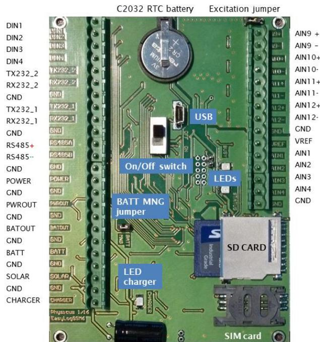
Thanks to clear layout the user can easily connect relatively large number of sensors. For better access to input connections, connectors are divided by two or three and removable.
