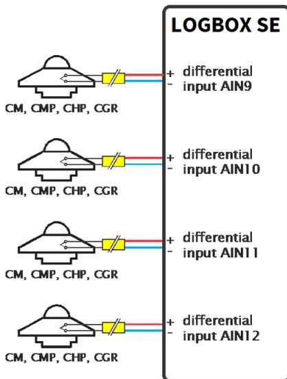
The LOGBOX SE allows you to connect up to 4 sensors on the differential analog inputs AIN9 to AIN12 which have a selectable input from 19mV up to 2500mV.
