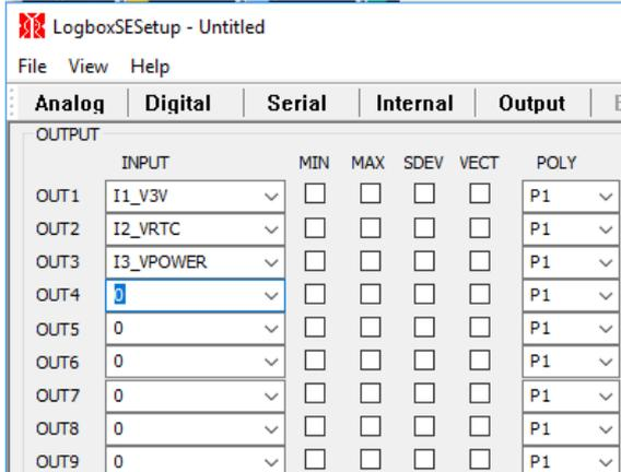
Using the Modbus® RTU protocol and function 4 “Read Input Registers” one can retrieve actual data from the registers. The registers start at 100 and with 32 two byte registers it goes to 163.
