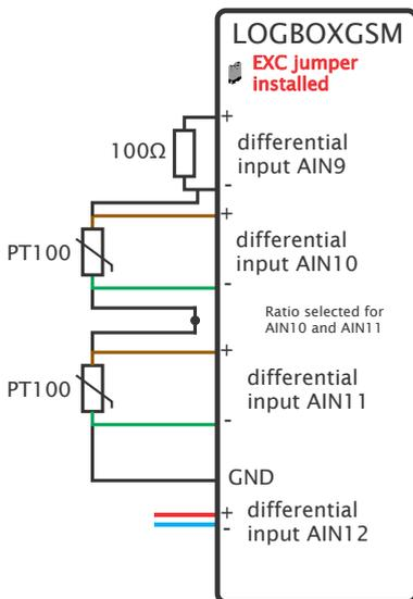
The ratio selection in the analog setup page can take care of the calculations needed. Range should be 78mV. Select Ratio for **both** AIN10 and AIN11.
