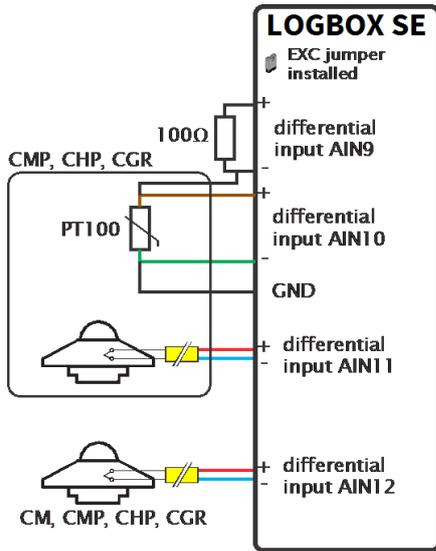
The LOGBOX SE allows you to connect one Pt-100 temperature sensor:
