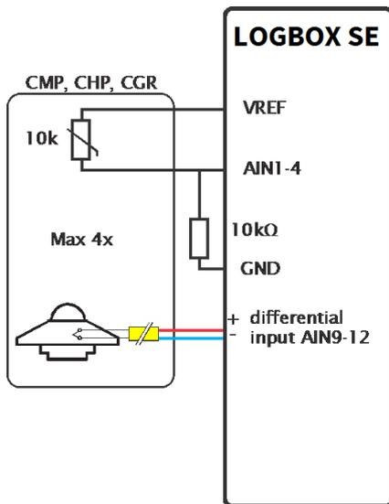
In the illustration the 10K thermistor is connected to AIN 1 but in practice it can be connected to any of the four analog single ended inputs AIN1 – AIN4.
