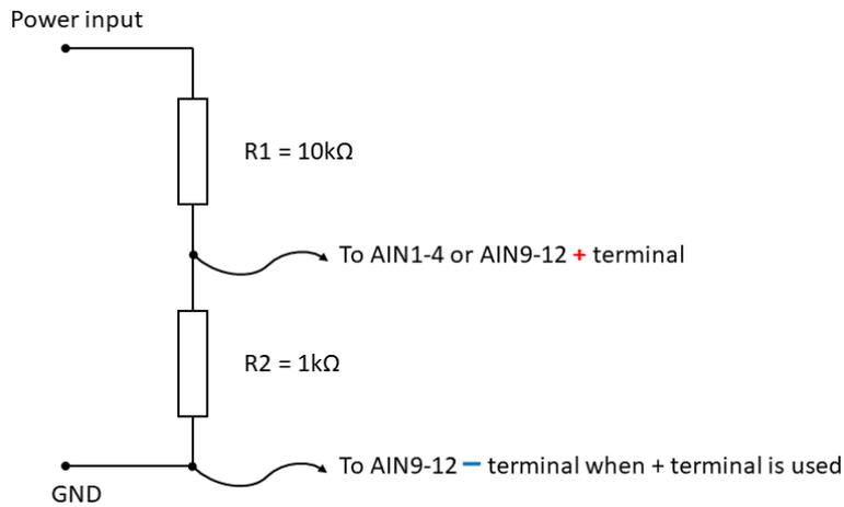
Input range 2500mV for the differential inputs.
