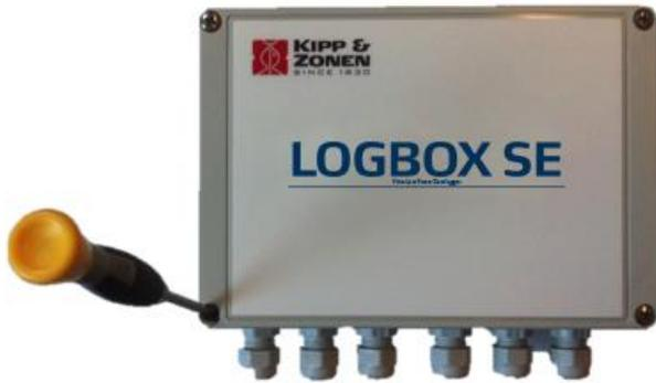
With the switch in Off position now connect a power supply in the range of 4...20Vdc to POWER or CHARGER or the lead acid battery to BATT. For mobile power supply there is the holder for six AA type batteries that needs to be connected to POWER with the BATT jumper removed for the lowest power consumption possible.
