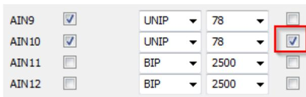
It's designed for Pt-100 measurements, where AIN9 is connected to a high precision 100ohm reference resistor and AIN10 is connected to Pt-100 sensor. This way the user can measure temperature with 4 wire method (for highest precision).
