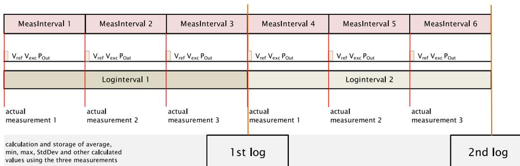
RepInterval [0...3600] – interval between reports in seconds on COM2 serial port. If RepInterval is zero, there is no report on COM2. If RepInterval is non zero and equal to LogInterval, reports on COM2 will be the same as logged data. If RepInterval is non zero and different from LogInterval, reports on COM2 are generated from last measured data (without min, max, stdev).
