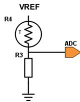
**Standard polynomials** for 10k thermistor to  $V_{REF}$ , 10k resistor to GND
