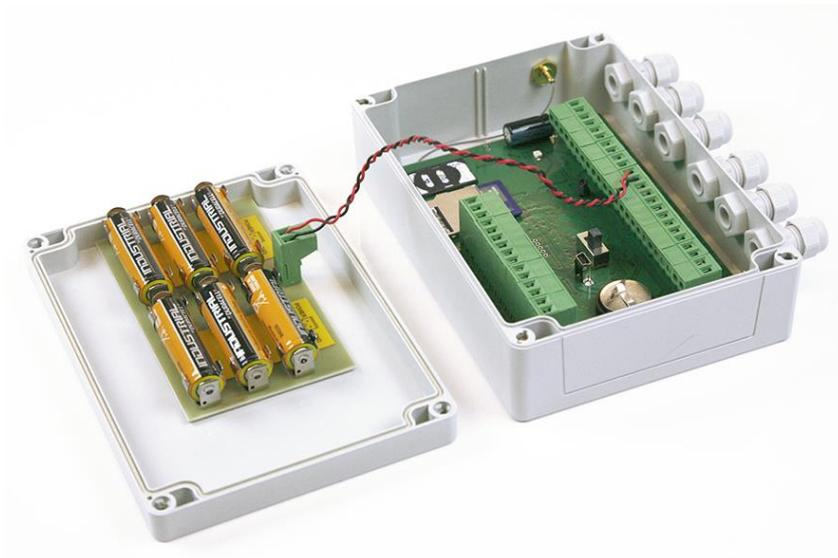
Last step is to connect the supplied USB cable with the computer. The LOGBOX SE Setup software can be used to setup the logger and related sensors. Do not switch the LOGBOX SE on yet. The USB connection or 6 AA batteries can both supply the board enough electrical power to perform the setup.
