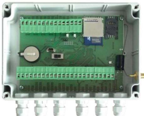
▲The original model with 2G GPRS modem
