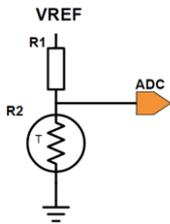
**Standard polynomials** for 10k thermistor to GND, 10k resistor to  $V_{REF}$
