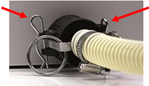
Figure 6: securing the Camlock
