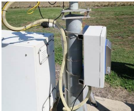
Figure 7: Example of mounting the air supply cabinet
