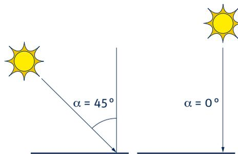
Ideally a pyranometer has a directional response which is exactly the same as the cosine-law. However, in a pyranometer the directional response is influenced by the detector and by the quality, dimensions and construction of the dome(s). The maximum deviation from the ideal cosine-response of the pyranometer is given up to  $80^\circ$  angle of incidence with respect to  $1000 W/m^2$  irradiance at normal incidence ( $0^\circ$  zenith angle).
