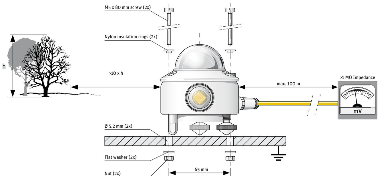
**Note** After recalibration and/or reinstallation ensure that the nylon insulators are refitted.
